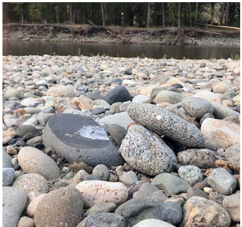
A tracer stone on a gravel bar in the Methow River. The small white spot on the rock at the center of the photo is the epoxy used to seal the PIT tag inside the rock.
